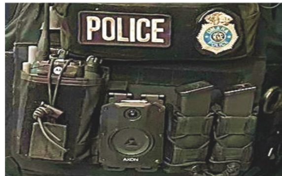
Picture of an Axon Body Worn Camera on an officer's vest. The device in the middle is the camera.
