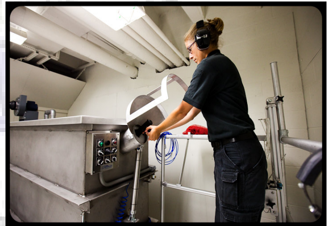
Crime Lab Tech Molly Claus fires a handgun for a ballistics test (Photo courtesy of Timothy Keen)
